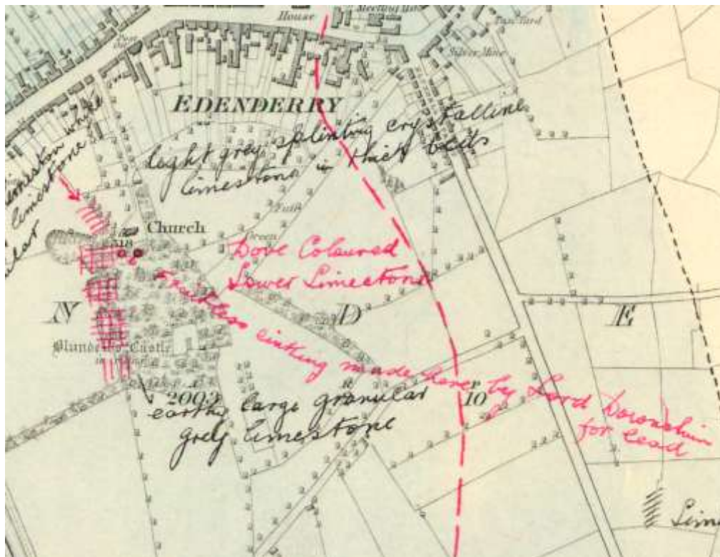
Figure 5. Fair copy geological field map (circa 1850's) showing three shafts and note "Fruitless working made here by Lord Downshire for lead"
