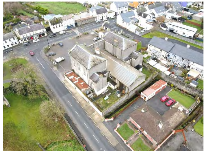
Aerial view from drone survey, north to top right of page Note metal sheet roofs to central auditorium and southern single storey extension.
