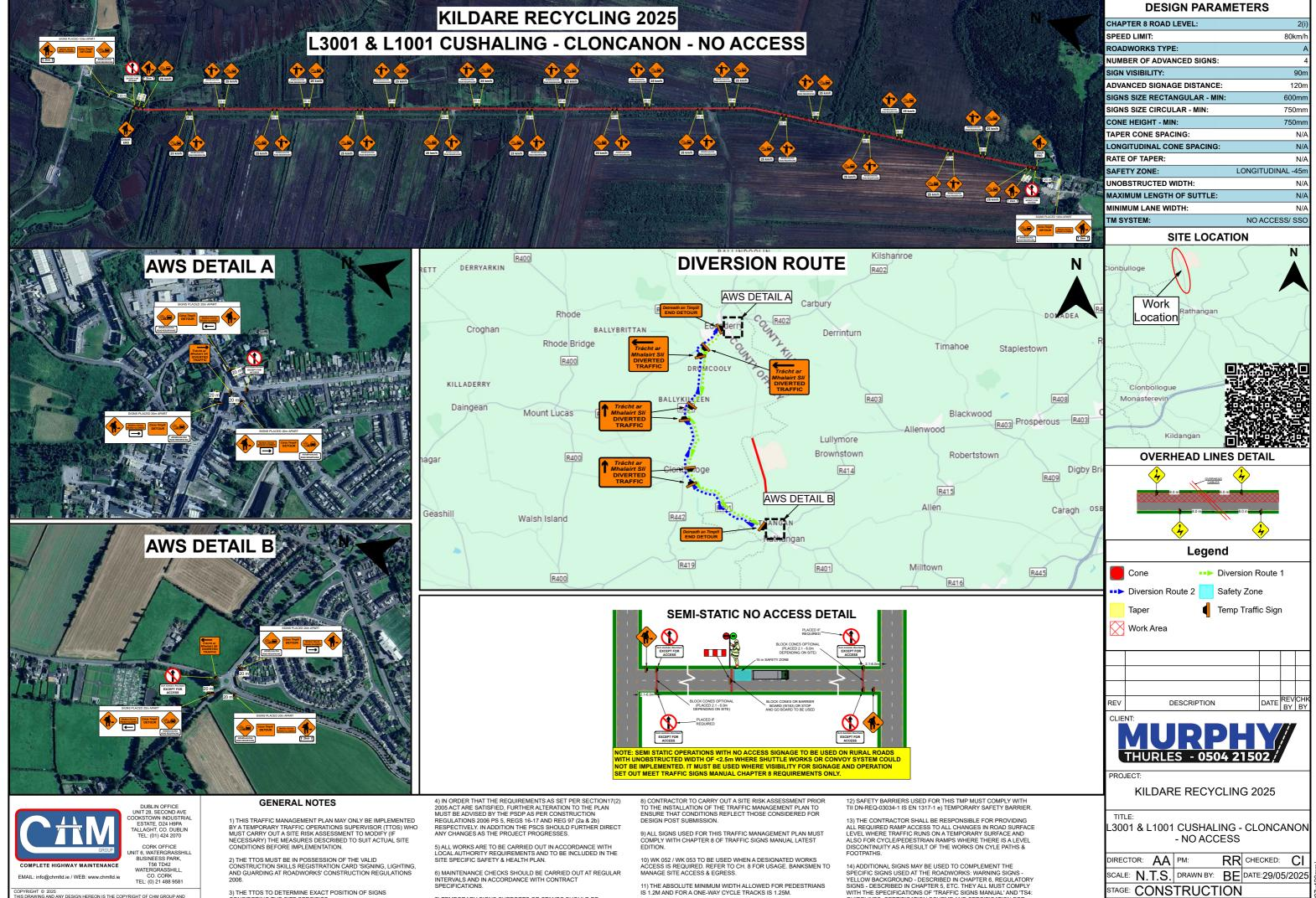
7) TEMPORARY SIGNS SUPPORTS OR STANDS SHOULD BE DESIGNED IN ACCORDANCE WITH SPECIFICATION TS4.
