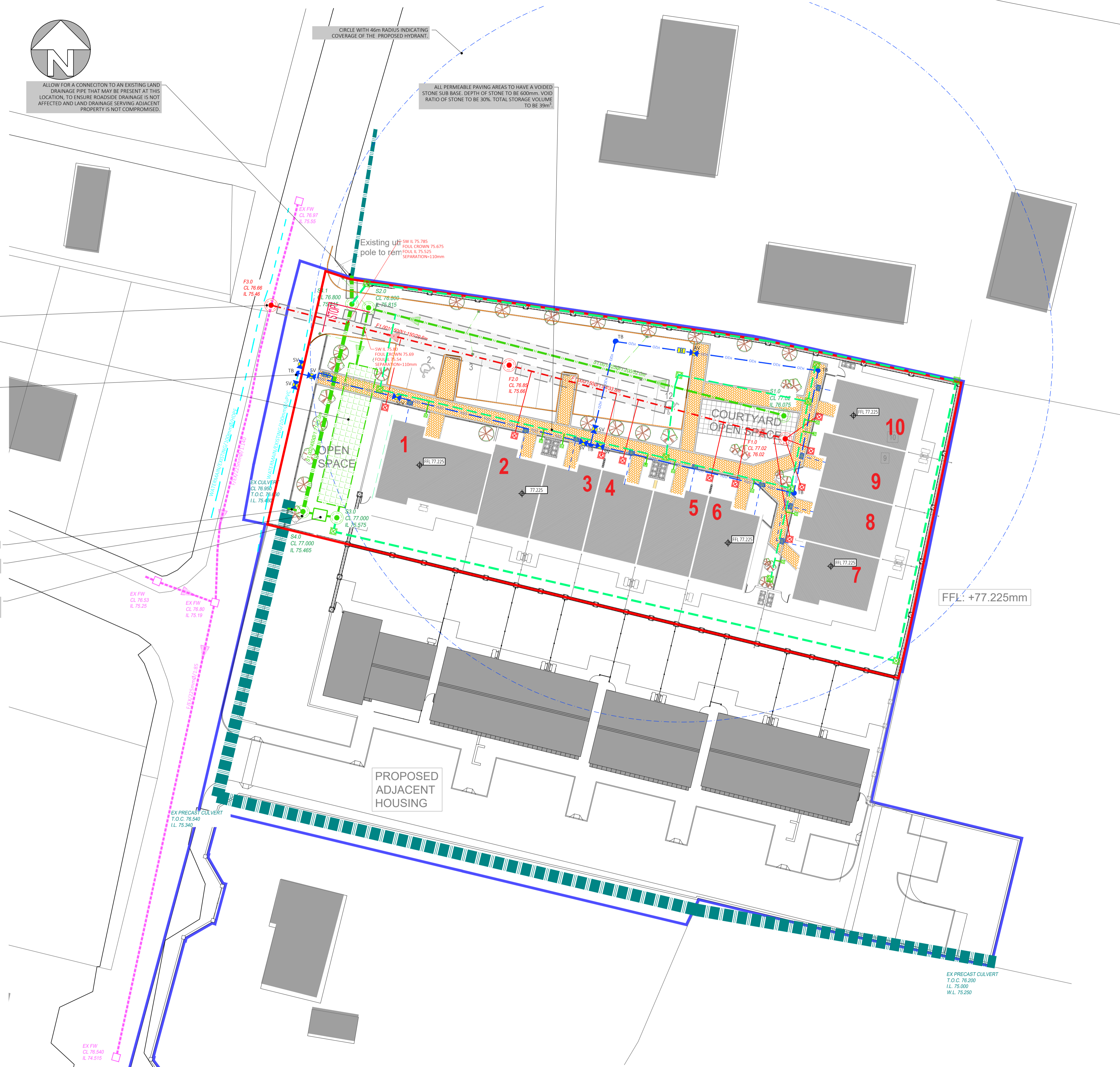
SITE LAYOUT PLAN - PART PLAN 1 - SERVICES - WASTEWATER, SURFACE WATER & WATERMAIN
