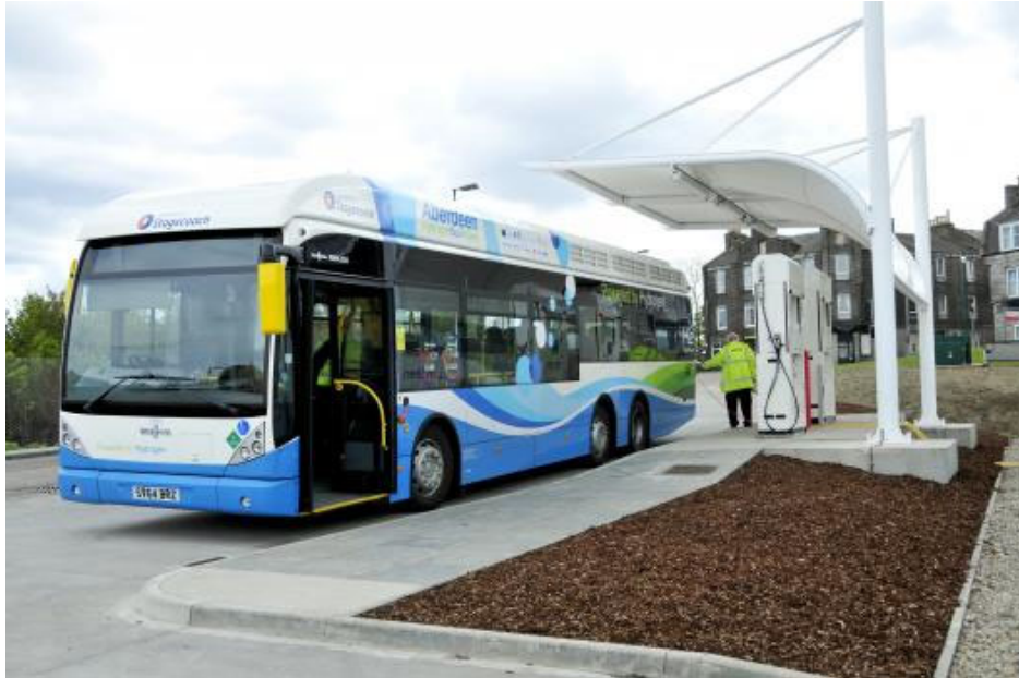
Figure 4-16: Hydrogen Fuel Cell Bus refuelling in Kittybrewster, Aberdeen
