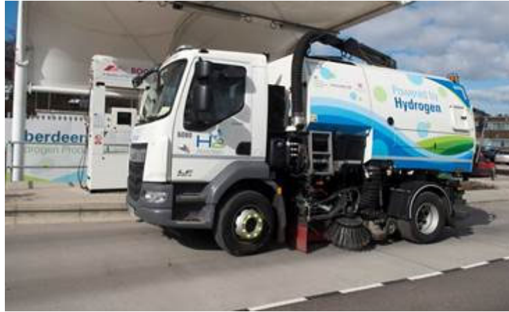
Figure 4-27: Road Sweep in Aberdeen converted to diesel / hydrogen ‘dual fuel’ operation (HyTIME Project / H2 Aberdeen)
