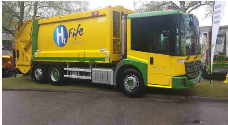
Figure 4-22: Waste Collection Vehicle (WCV) in Fife converted to diesel / hydrogen ‘dual fuel’ operation
