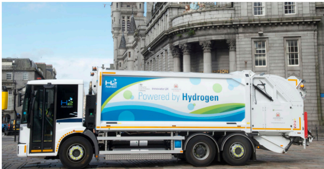
Figure 4-26: Waste Collection Vehicle in Aberdeen converted to diesel / hydrogen ‘dual fuel’ operation (HyTIME Project / H2 Aberdeen)
