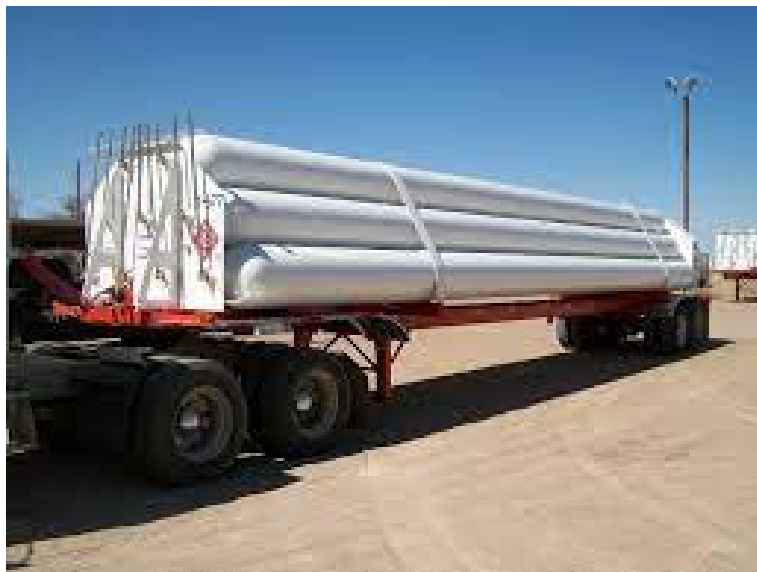
Figure 3-4: Tube Trailer for transporting Compressed Hydrogen Gas at 350bar
