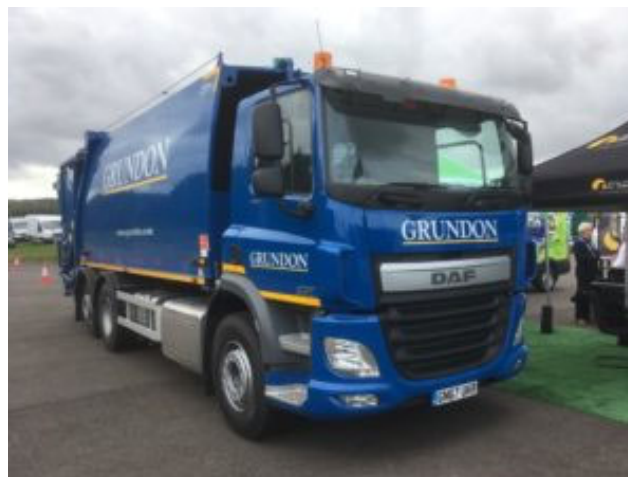
Figure 4-28: Waste Collection Vehicle (WCV) in Oxfordshire converted to diesel / hydrogen ‘dual fuel’ operation
