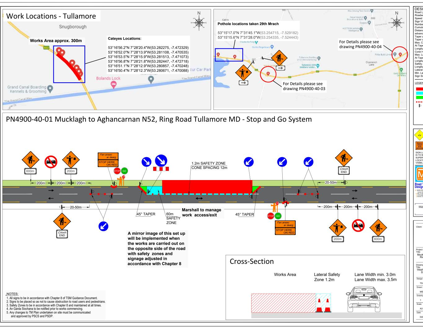
DESIGN PARAMETERS Roadworks Type Speed Limit Sign Visibility Number of Signs - 120m Cumulative Distance - 600m Distance between advance signs (m) - 200m Taper at Lane Taper at HS - 1 in 60 - 1 in 30 Max. Cone Spacing: At Tapers - 3m Longitudinal - 12m 1000m Max. Lamp Spacing At Tapers Longitudinal Safety Zones: - 24m Longitudinal - 60m Lateral - 1.2m Min. Lane Width - 3.0m - 750mm LEGEND: WORKS AREA SAFETY ZONES TAPER • • • CONES SIGN LOCATION
